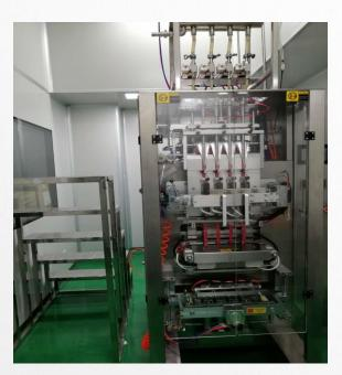
Packing machine for Liquid preparation
